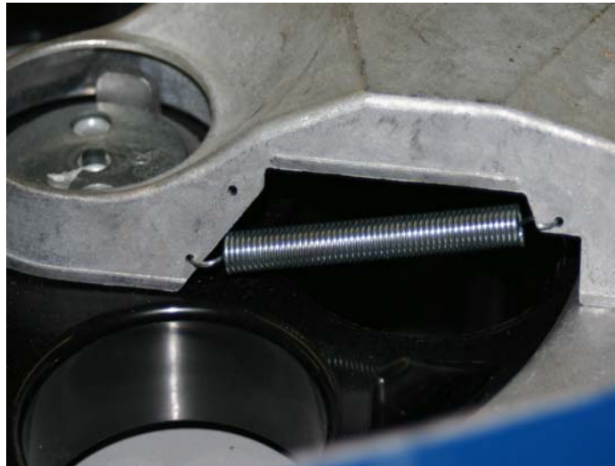
Proper brush off spring position to properly dispense 45mm, 49mm and 2" capsules.
